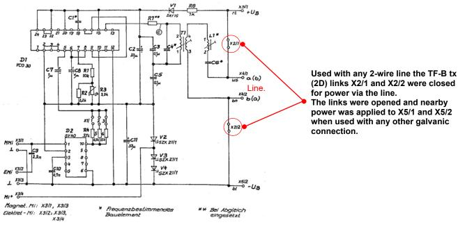
Circuit diagram of TF-B tx (2D) bug. Either a electro magnetic or a electret microphone could be connected.
