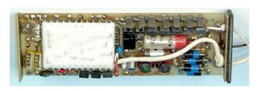
Top view of TF-B tx (2D) board. The microphone amplifier chip D2 (SV40) was hidden under the PLL chip D1 (VCO30).
