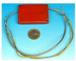
TF-B tx (2D) covert number 31115-122, earlier model with external microphone known as 'Leipzig alt flach (old flat) 24V'.
